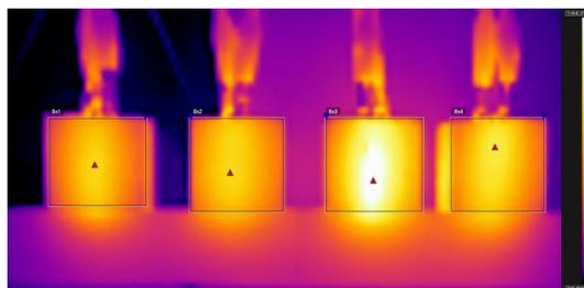
Fig. 1 Thermal image of voltage-connected ECCCs
